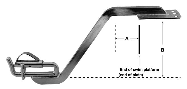
A \_\_\_\_\_\_ The distance from the outside edge of the swim platform to the point where the offset starts angling down: MAXIMUM - 4"
