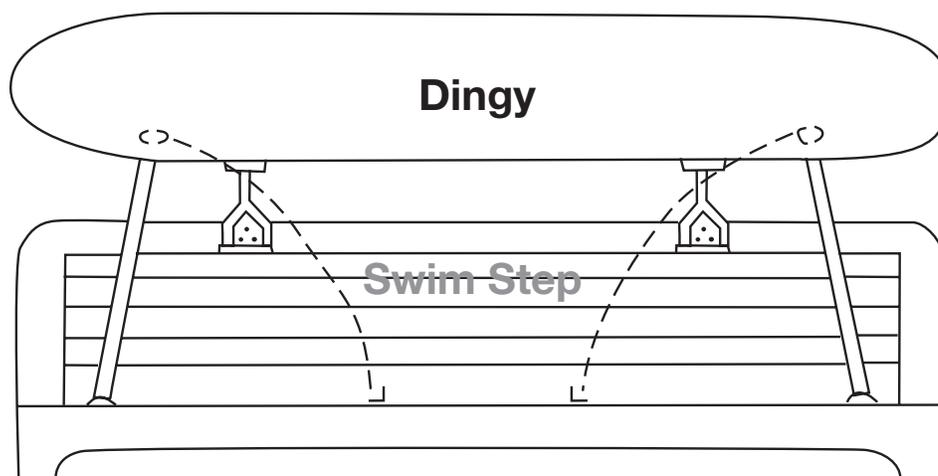
**Step 1** — Mount the brackets at a 10:00 and 2:00 o'clock position. This will provide rigidity for the dinghy. See above figure.
